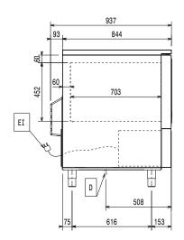
Drain Electrical inlet (power)
